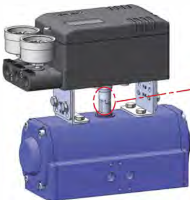
NAMUR Type Mounting ( VDI/VDE 3845, IEC 60534-6-2 )
